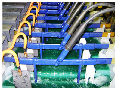
Quick Disconnect, User-Friendly Cathode Connection
