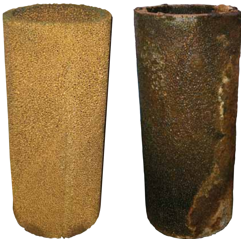
Above, a before and after look at PMPC’s “Gold Bug” system, which uses a metallic matrix of surface area in a cylindrical cathode. Below, combined with the turbulence created by a dedicated pumping system, it exposes the cathode to a continuously renewed concentration of fresh ions.
