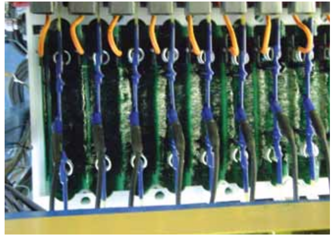
Metal is extracted as it is deposited in an electroplating process onto the cathode.
