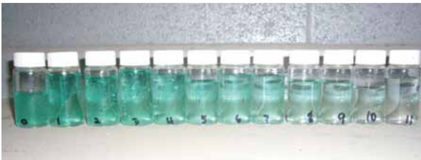
A comparison of hourly samples while electrowinning. Metallic ions are removed from concentrated rinse water and spent process solutions.
