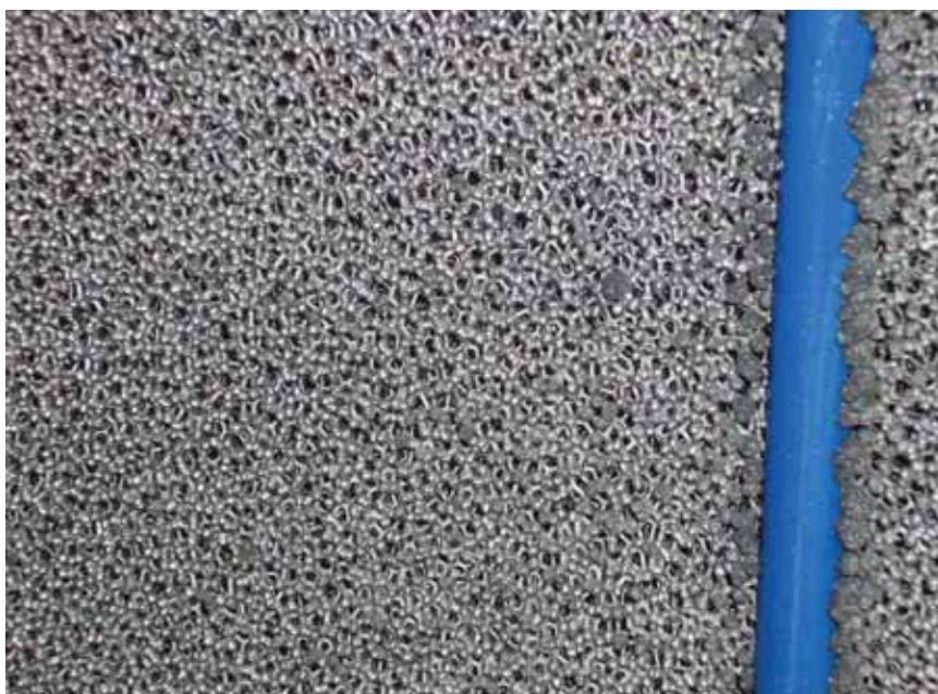
Above, a before and after look at PMPC’s “Gold Bug” system, which uses a metallic matrix of surface area in a cylindrical cathode. Below, combined with the turbulence created by a dedicated pumping system, it exposes the cathode to a continuously renewed concentration of fresh ions.
